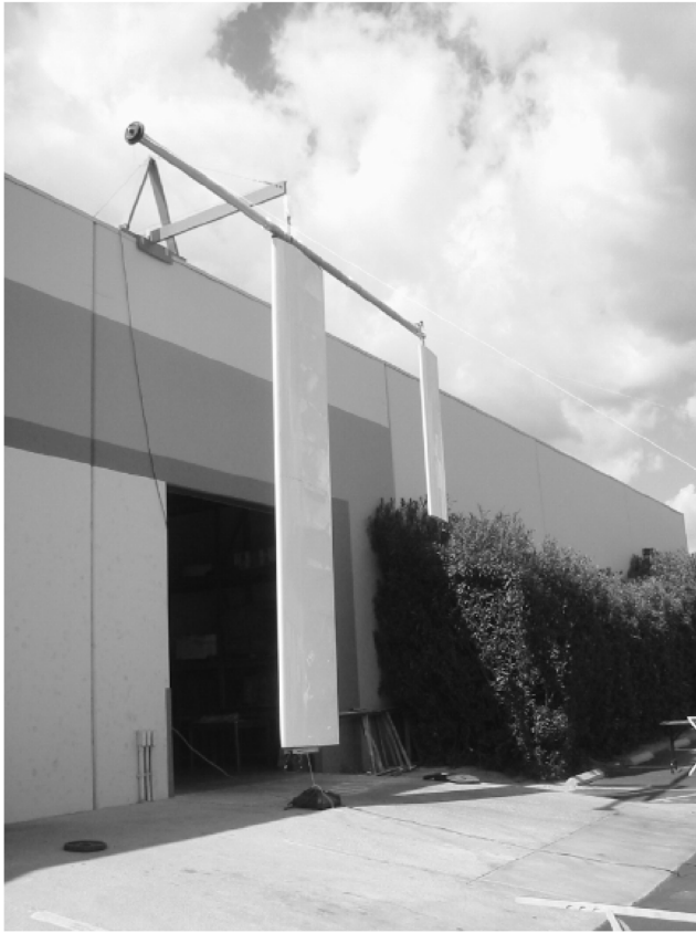
Fig. 1 Full-scale mechanical prototype winged balloon guidance system.
